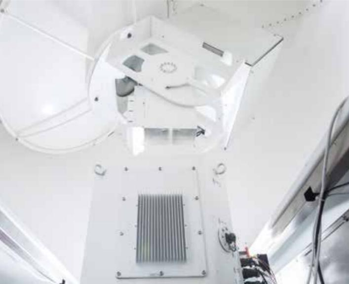
The system compasses a magnetron-based transmitter and employs coherent-on-receive techniques to obtain high resolution in both Range and Doppler. But the system-level design has been carried out under the requirement of an easy transition to solid-state-based transmitter, if requested. Both transmit and receive RF chains possess automatic or user-initiated dynamic calibration topologies in amplitude and phase to minimize ZDR and  $\text{ØDP}$  errors.
